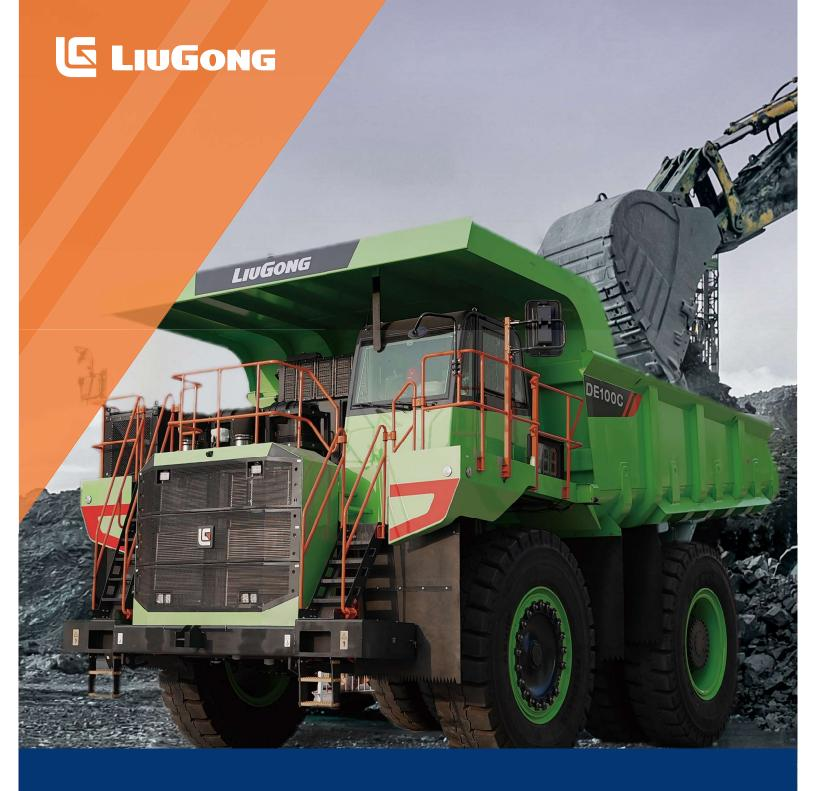
Max. Gross Machine Weight169,000 kgNet Machine Weight72,000 kgPayload97,000 kgEngineCummins M15×2Rated Power1126 kW (1510 hp / 1531 ps) @ 2,100 rpmMax. Speed55 km/hStruck Capacity46 m³Heaped Capacity (SAE 2:1)63 m³
